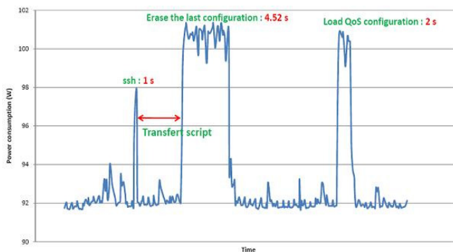
Fig. 4. Energy consumption when the router configuration is loaded manually and step by step.
